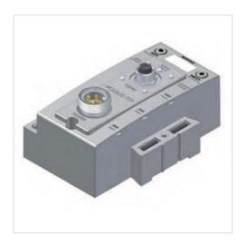
Ambient temperature min./max. -10 ... 50 °C 24 V DC Operational voltage electronics Electronics voltage tolerance -10% / +10% Power consumption electronics 0.03 A 24 V DC Operating voltage, actuators Total current for actuators 4 A Protection class IP65 32 Number of valve positions max. Diagnosis Undervoltage
