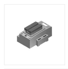
Version I/O module version Ambient temperature min./max. -10 ... 50 °C Operational voltage electronics 24 V DC Electronics voltage tolerance -10% / +10% 0.05 A Power consumption electronics Power supply for actuators 24 V DC 4 A Total current for actuators Protection class IP65 Total current of sensors max. 1,2 A Diagnosis Short circuit
