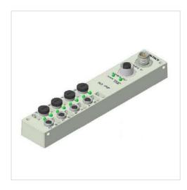
Version I/O module version -10 ... 50 °C Ambient temperature min./max. Operational voltage electronics 24 V DC Electronics voltage tolerance -10% / +10% 55 A Power consumption electronics Max. current per channel 0.15 A 24 V DC Power supply for actuators Total current for actuators 4 A Protection class IP65 Total current of sensors max. 1,2 A Diagnosis Short circuit
