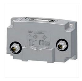
Version Bus coupler Ambient temperature min./max. -10 ... 50 °C Operational voltage electronics 24 V DC -10% / +10% Electronics voltage tolerance Power consumption electronics 0.1 A 24 V DC Operating voltage, actuators Total current for actuators 4 A Protection class IP65 32 Number of solenoid coils max. Number of valve positions max.
