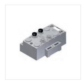
Version I/O module version -10 ... 50 °C Ambient temperature min./max. Power consumption electronics 55 A Max. current per channel 0.15 A 24 V DC Power supply for actuators Total current for actuators 4 A IP65 Protection class Total current of sensors max. 1,2 A Diagnosis Short circuit Weight 0.274 kg
