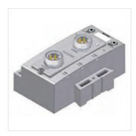
Version Bus coupler Ambient temperature min./max. -10 ... 50 °C Operational voltage electronics 24 V DC -10% / +10% Electronics voltage tolerance Power consumption electronics 0.11 A 24 V DC Operating voltage, actuators Total current for actuators 4 A Protection class IP65 32 Number of solenoid coils max. Number of valve positions max. 32 Undervoltage
