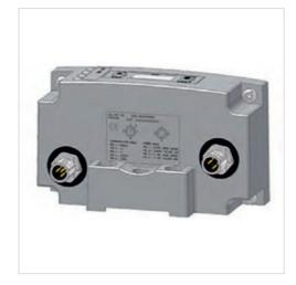
Ambient temperature min./max. -10 ... 50 °C 24 V DC Operational voltage electronics Electronics voltage tolerance -10% / +10% Power consumption electronics 0.1 A Operating voltage, actuators 24 V DC Total current for actuators 4 A IP65 Protection class Number of solenoid coils max. 32
