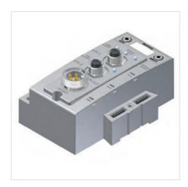
Version Bus coupler Ambient temperature min./max. -10 ... 50 °C Operational voltage electronics 24 V DC -10% / +10% Electronics voltage tolerance Power consumption electronics 0.104 A 24 V DC Operating voltage, actuators Total current for actuators 4 A Protection class IP65 Number of solenoid coils max. 128 Number of valve positions max. 110 Undervoltage
