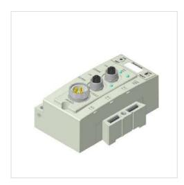
Version Bus coupler Ambient temperature min./max. -10 ... 50 °C Operational voltage electronics 24 V DC -10% / +10% Electronics voltage tolerance Power consumption electronics 0.11 A 24 V DC Operating voltage, actuators Total current for actuators 4 A Protection class IP65 Diagnosis Undervoltage I/O module extension max. 16
