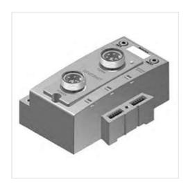
Version Bus coupler Ambient temperature min./max. -10 ... 50 °C Operational voltage electronics 24 V DC -10% / +10% Electronics voltage tolerance Power consumption electronics 0.11 A 24 V DC Operating voltage, actuators Total current for actuators 4 A Protection class IP65 32 Number of solenoid coils max. Number of valve positions max. 32 Diagnosis Undervoltage I/O module extension max. 16
